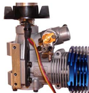
Figure 3. RPM sensor mounted on motor
